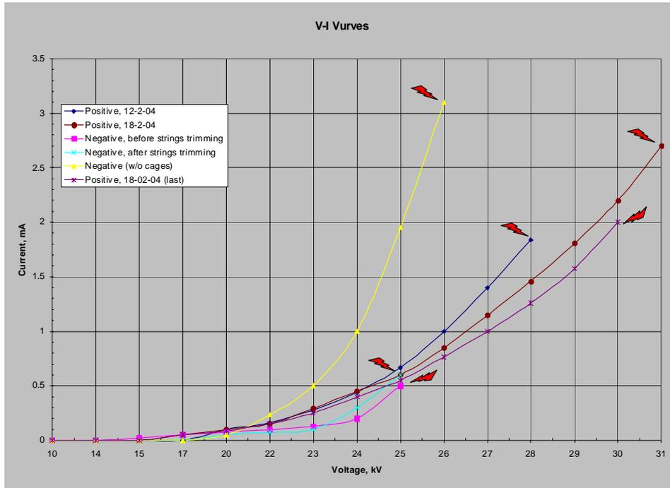
Figure 8 presents the results of the initial V-I characterization of the pilot MSC™. The initial tests were run in the positive corona mode, and the maximum voltage attainable prior to the onset of sparking was 28 kV. These initial tests were run with the hopper, inlet, and all inspection panels removed so that the areas of sparking could be identified and subsequently addressed. Figure 9 illustrates the sparking phenomena occurring between a discharge electrode and a plate.
