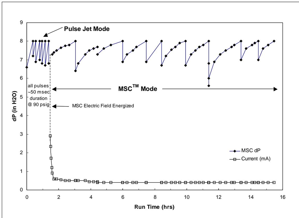
Figure 12 shows the pressure drop results for both sets of tests. With the electric field off, the pressure drop increased at a rapid rate, reaching 8.0 inches H<sub>2</sub>O in less than one hour. In
