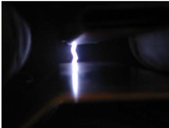
Following optimization of the electrical clearances, the maximum achievable voltage increased to 30 to 31 kV as shown by the positive corona results. Subsequent to optimizing the pilot unit in the positive corona mode, a series of tests were also run where a negative voltage was applied to the plates. As shown in Figure 8, sparking occurred at lower voltages in the negative corona mode.
